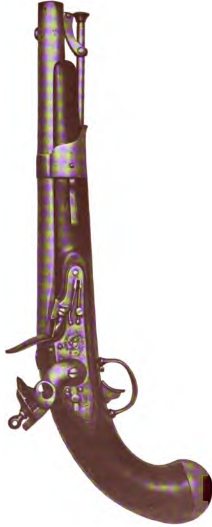
Horse pistol; model of 1819. Length 15 \frac{3}{4} inches. Length of barrel 10 \frac{1}{4} inches. Caliber, 54. Swivel ramrod. Sight on barrel. Iron mountings.
